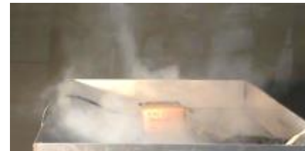
Gel packs prevented jets of sparks and flames from exiting box. Only cell experiencing thermal runaway vented.
