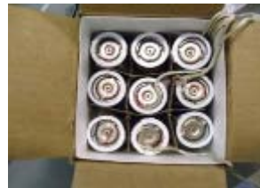
Gel packs prevented jets of sparks and flames from exiting box. Only cell experiencing thermal runaway vented.
