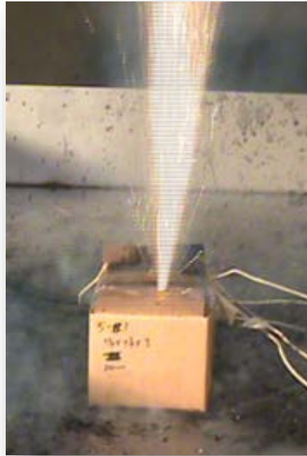
Thermal events - sparks and flames blow through box
