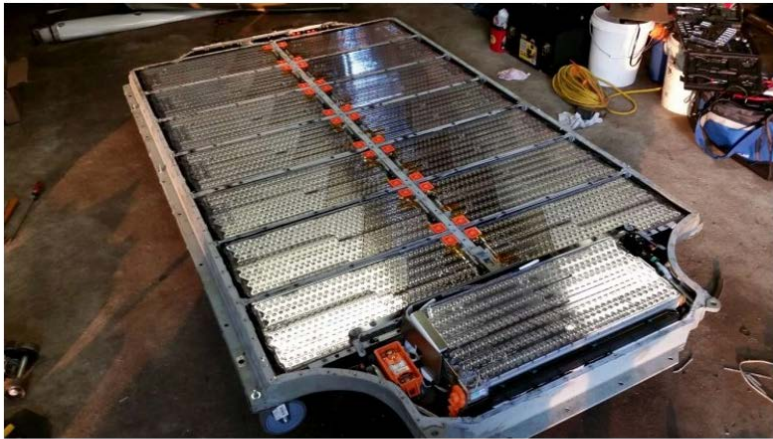
FIGURE 1.23 TESLA MOTOR'S BATTERY PACK, CONSISTING OF MORE THAN SEVEN THOUSAND OF 18650 CYLINDRICAL CELLS
