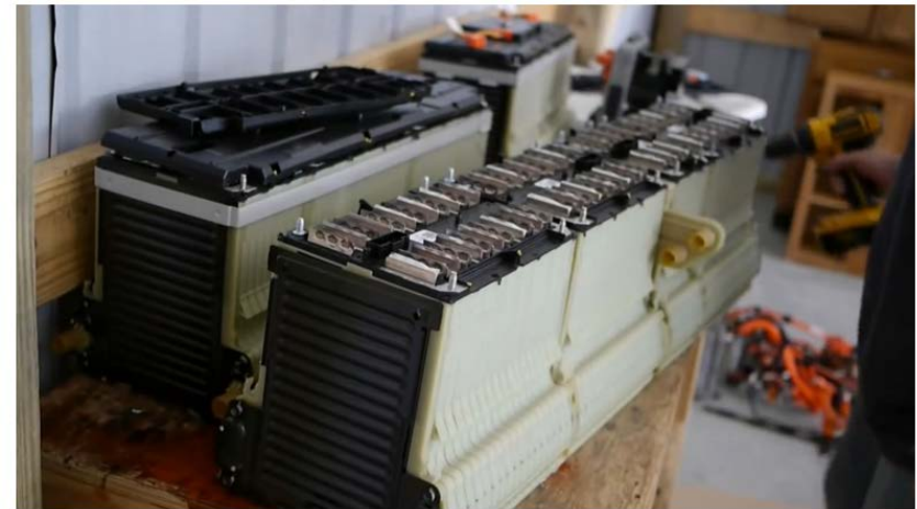
FIGURE 1.24 GM CHEVY VOLT: BATTERY MODULES WITH ULTRASONIC WELDS
