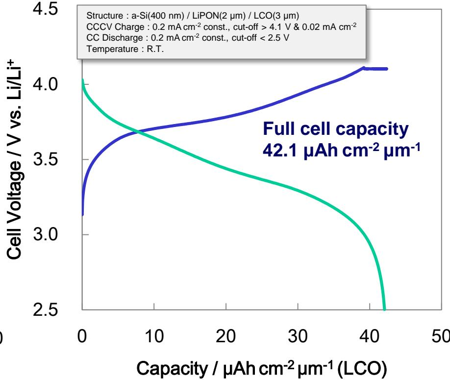
TFB with a-Si anode is formed by optimizing thickness ratio between cathode and anode.
