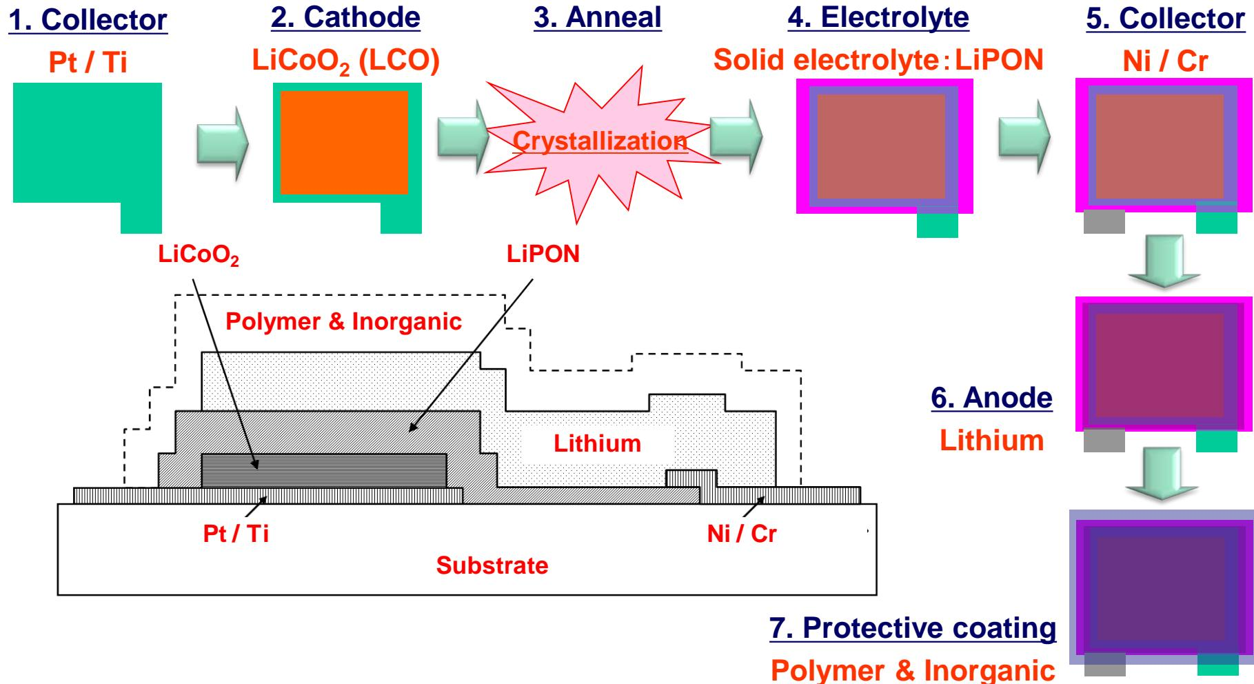
All layers are deposited using mask for patterning.
