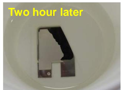
Vigorous reaction of Li and water cannot be seen and reaction proceeded slowly from cracked part.
