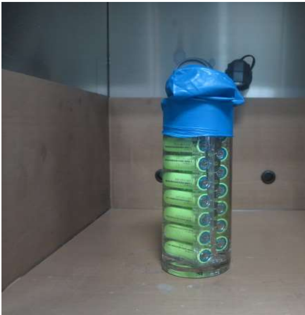
0.28KWh battery module soaked in clear water
